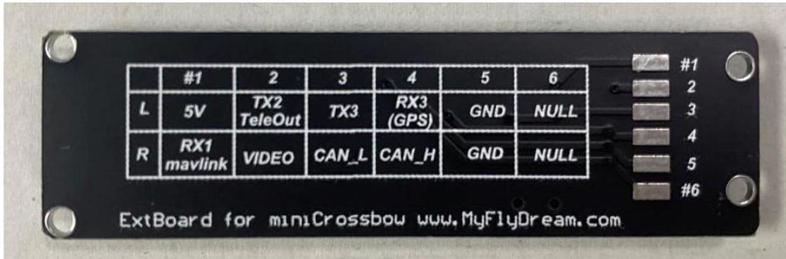
The "L" row matches the LEFT port. Pin1=5V, Pin2=TX2, Pin3=TX3, Pin4=RX3, PIN5=GND.
