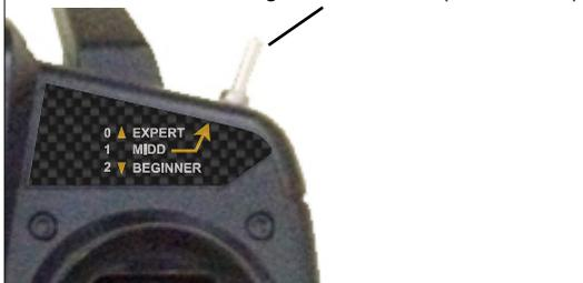
The airplane comes with pre-installed X-PILOT to help control flying easily. The switch is with 3 levels to control the X-PILOT. To turn on the X-PILOT, switch to upper position(towards you). To turn off the X-PILOT, switch to lower position(away from you).
