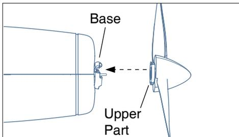
The propeller saver keeps the propeller from damage, and prevent the electronic components from over current. When the airplane hits any obstacle, the propeller will loose from the base. To install the propeller back to the base, insert the upper part centerly through the motor shaft, and hearing a "click" sound to ensure it is secured.
