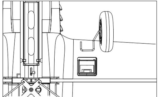
2. Plug the landing gears into the position on the mainwing as shown above.
