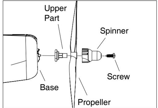
Follow below steps to replace broken propeller and shaft adaptor. You will need help of a Philips screw driver and pliers(not included).
