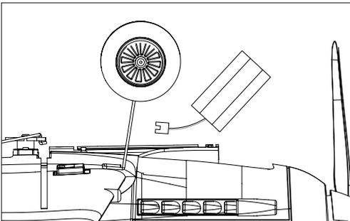
3. Connect the battery to the receiver, then stick the battery into the cabin.
