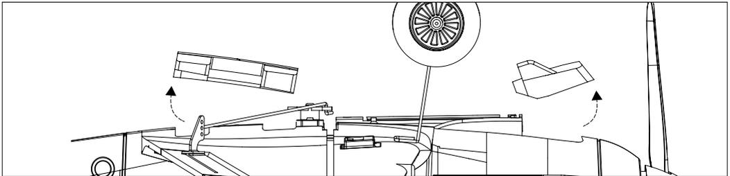
1. Take off the cover in the head of fuselage to replace the motor, or the cover in the middle of fuselage to replace the receiver. It is no need of tool to take off the covers.
